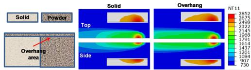
Figure 2. Thermal response from simulations of EBAM-fabricating an overhang part.
