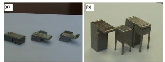
Figure 10. (a) Fabricated overhang parts using heat supports with different gap distances, from Left to Right: 7, 9, and 11 layers. (b) Overhangs with heat support of different thicknesses: 10 mm (left) and 5 mm (right).
