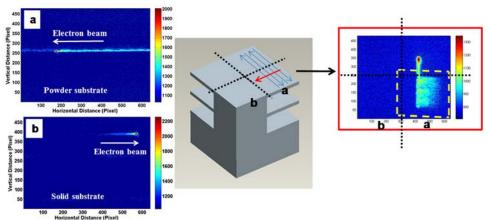
Figure 3. Thermal images from building overhang-type features, showing drastically different temperature distributions between scanning on a solid substrate and on an overhang.
