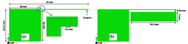
Figure 5. Overhang model geometry used in simulations: (a) without and (b) with a heat support.
