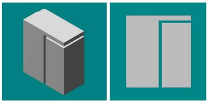
Figure 8. CAD model of an overhang part with a heat support.
