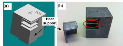
Figure 4. An example of (a) contact-free heat support in an overhang model and (b) the fabricated overhang without distortion.
