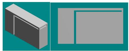
Figure 14. CAD model of a long overhang with heat support plus anchors.
