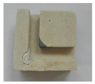
Figure 22 Cutaway of the trimaterial sand mold
