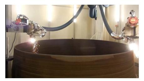
Figure 6. DMD simultaneous dual nozzle printing of the RS-25 liner.
