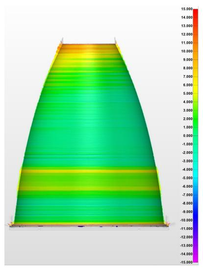
Figure 8. 3D scanned data overlayed on the CAD of the part showing dimensions of the DMD printed part.
