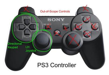
Figure CG-1 - The controls that are circled in green on the PS3 Controller pictured above must be fully operable by the adaptive device. The buttons with red "X"s through them do not need to be operated.
