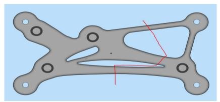
Figure MC-9: The fracture path that Team Member C identifies when twisting the part.
